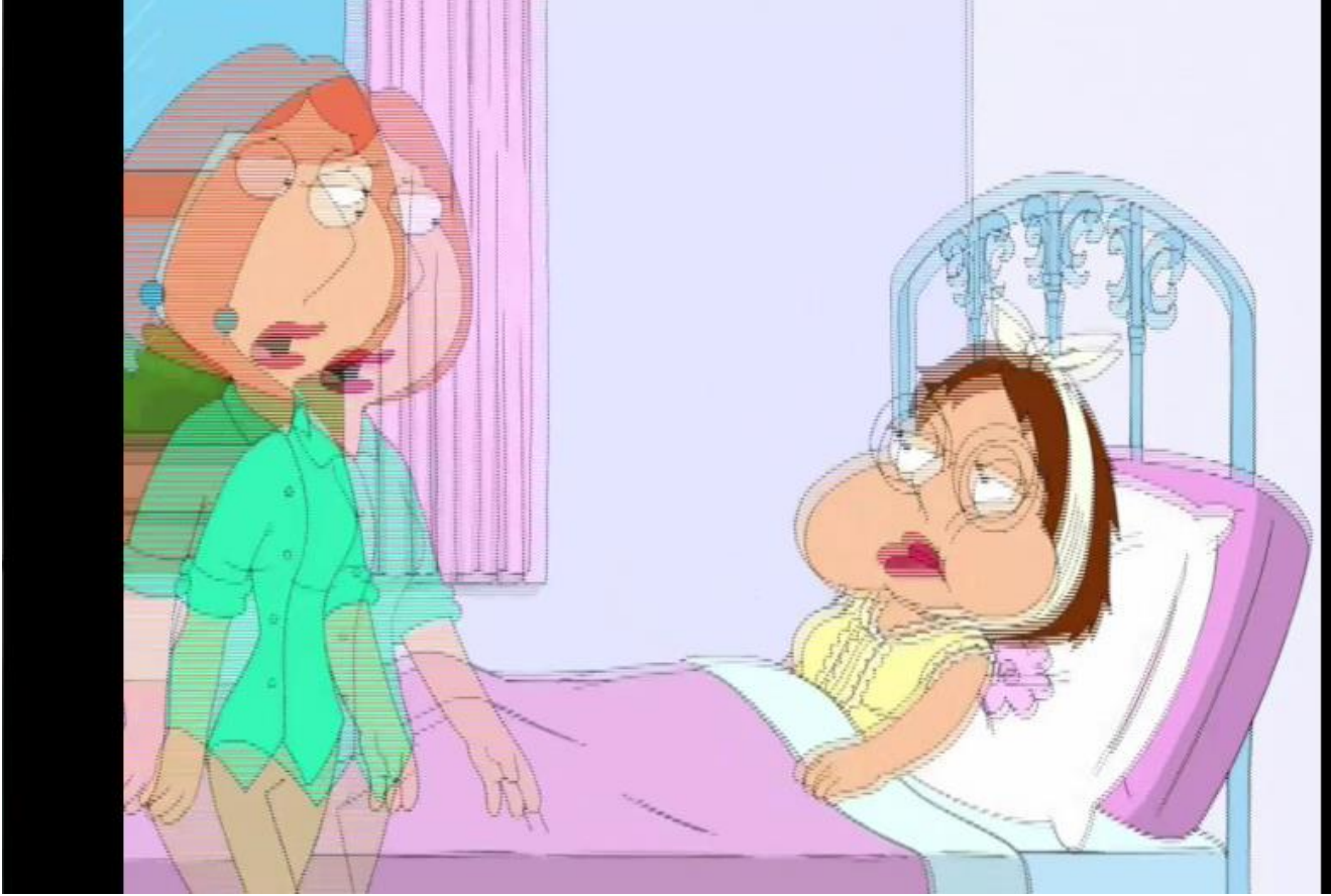
Unacceptable 3-2 pulldown errors showing double image frames
